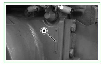
PY28290-UN: Transmission serial number LEGEND: A - Transmission Serial Number Plate
