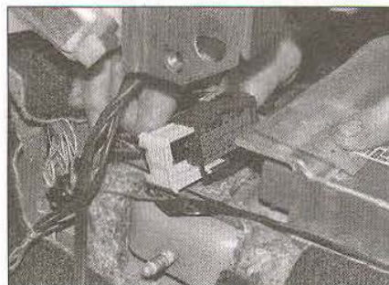
26.45 Open the locking bar and disconnect the wiring harness connector at the front of the airbag control unit
