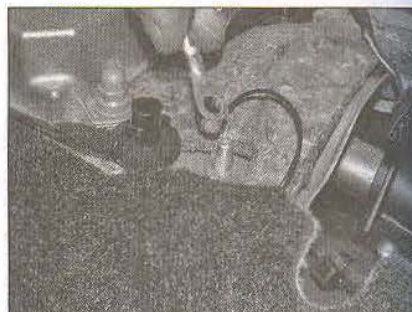
26.46a Undo the nuts and disconnect the earth lead behind the airbag control unit ...
