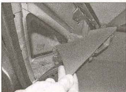
26.35 Unclip and remove the fascia upper end panels on both sides
