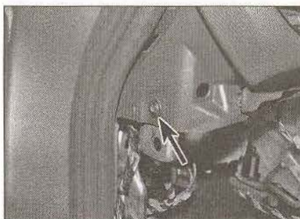
26.37a Undo the bolt (arrowed) at the left-hand and right-hand end of the fascia ...
