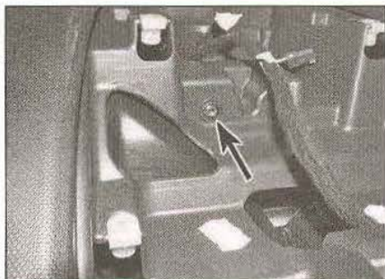
26.37c ... and the bolt (arrowed) in the fascia centre switch/vent panel aperture
