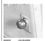
Depress brake pedal(s) and engage service park brake lock.
