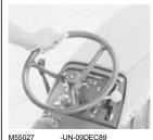
Count the number of revolutions of the steering wheel from a full right turn to a full left turn then, from a full left turn to a full right turn.
