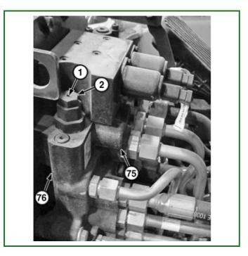
TX1250641A-UN: Hydraulic System Relief Valve
