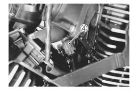
• Disconnect the ignition coil/plug cap lead wire couplers and remove the ignition coils/plug caps. ( 2-13 and -14)
