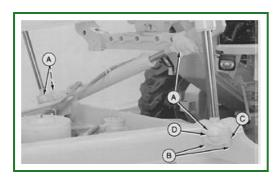
T6164BL-UN: Cylinder Ball/Socket Clearance—Adjust Shims LEGEND:
