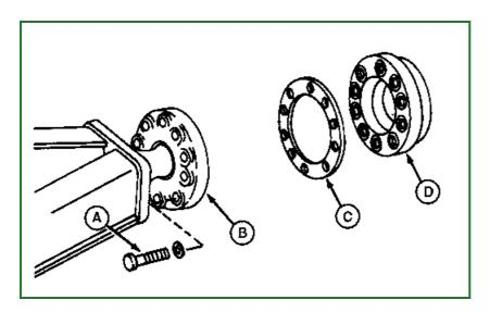
T107587-UN: Draft Ball Pivot Clearance—Adjust Shims
