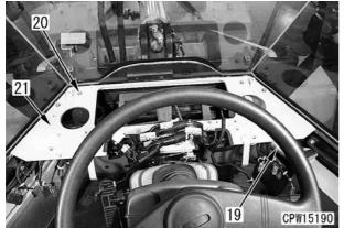
16. Remove 8 mounting bolts (20) and plate (21).
