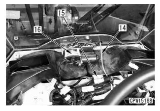
14. Remove left duct (17) and right duct (18).
