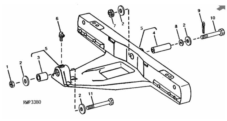
John Deere > Agriculture > TRACTOR > 4555 - TRACTOR > 4555, 4755, 4955 Tractors (North American Edition) (PC2270) > 80 Wheels, Front Axles and Sheet Metal > FRONT AXLE CENTER - ST469028
