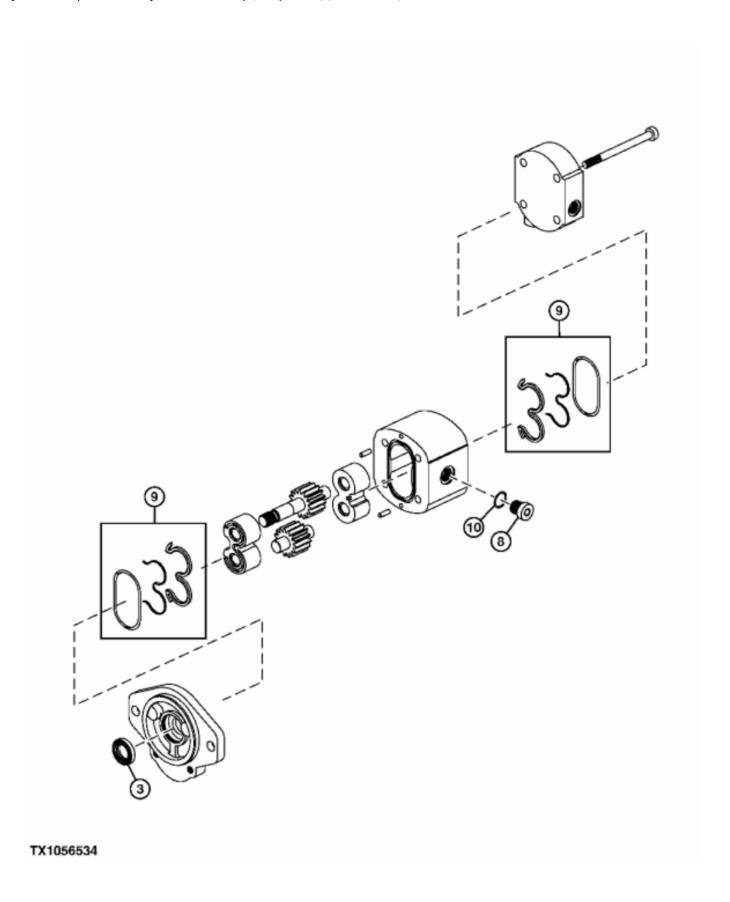
John Deere > Agriculture >LOADER, FOUR-WHEEL DRIVE >244J - LOADER, FOUR-WHEEL DRIVE >244J Loader (PC9370) >21 Vehicle Main Hydraulic System >2161 Hydraulic Pumps & Drives >Hydraulic Gear Pump (Components) (23290 - 35751) - ST39062
