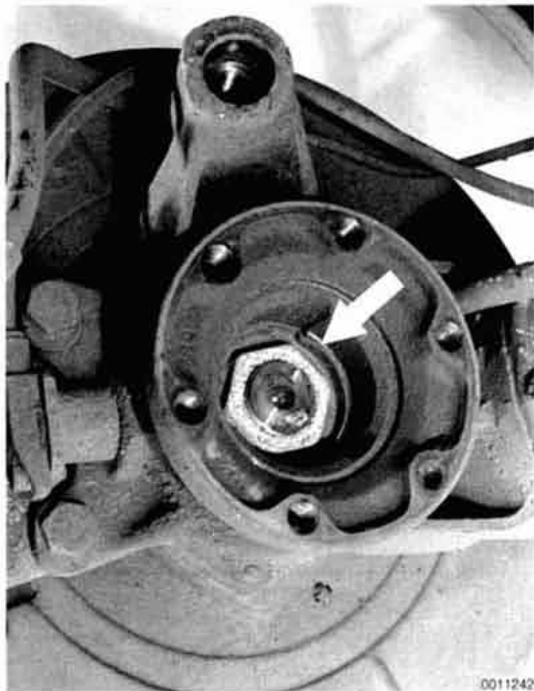
Fig. 7. Drive flange collar nut and lockplate (arrow).
