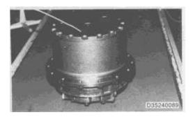
1. Remove plug (28) from the travel drive cover and let the oil drain from the travel drive. To facilitate oil draining, remove plug (27).
