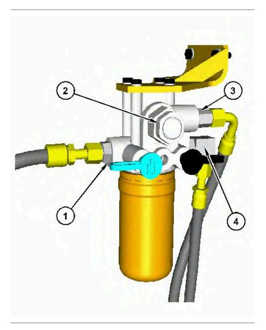
(1) Inlet port (oil flow from pilot pump)
