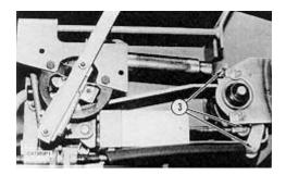
3. Mark and identify all lines and remove. Remove linkage (3).
