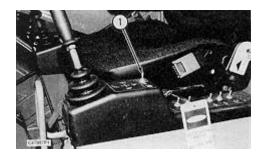
1. The engine speed control switch (1) is located to the left of the operator.
