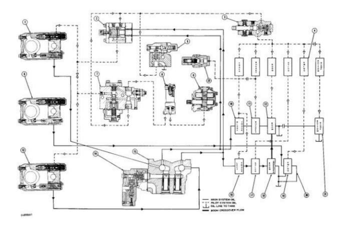
(1) Axial Piston Pump (Front). This is a variable displacement pump. It supplies the main oil flow to operate the right track motor, the bucket cylinder, the boom cylinders and the bottom dump cylinders when the machine is equipped with a bottom dump bucket (front shovel).
