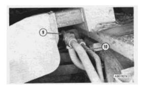
4. Tighten tubes (9) and (10) on the tee connector.
