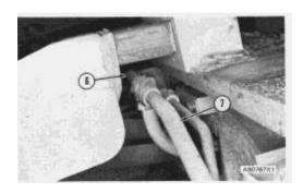
**4.** Loosen tubes (6) and (7) which are fastened to the tee connector.
