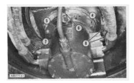
**3.** Use tooling (A) to lift the swivel into position. Make sure the six bolt holes in the rotor are in alignment with those in the manifold. Install eight bolts (4) which fasten the swivel to the undercarriage. Remove bolt (3) and tooling (A). Install tubes (5) and (6) on the swivel. Install the clamp (not shown) which fastens the tubes to the undercarriage. Install O-ring seals on four hoses (7) and (8). Install the four hoses on the swivel.
