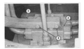
1. Remove two bolts (3) and remove arm (1) from manifold (2).
