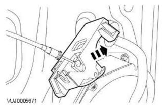
6. Remove the exterior door handle bezel retaining screw.
