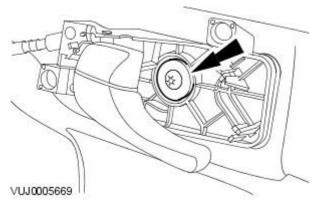
**4.** Release the actuator remote cable from the interior door handle.
